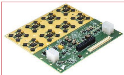
Fig. 1 A planar phased array front-end prototyping board (component side).
